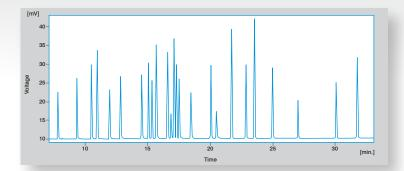
The packaging material monitoring is becoming one of the most important target in the food industry. Master SHS permits a complete automatic sampling and analytical system for the residual solvent determination acceding the minimum detectable levels below currently recommended by the norms (EN13628-2:2002).
