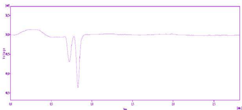
µTCD channel B chromatogram of the Gas standard mixture. It is possible to see the peaks of Helium and H2.
